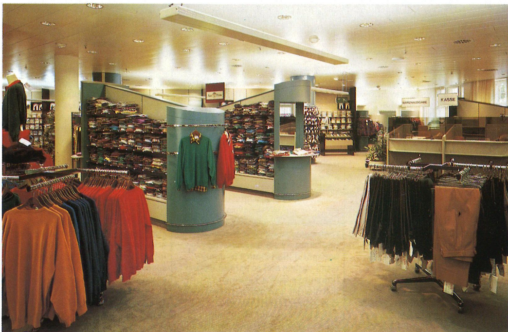
Compact metal-halide lamps produce a distinct beam with high luminous efficacy and excellent colour rendering which is ideal for this men's clothing department.
