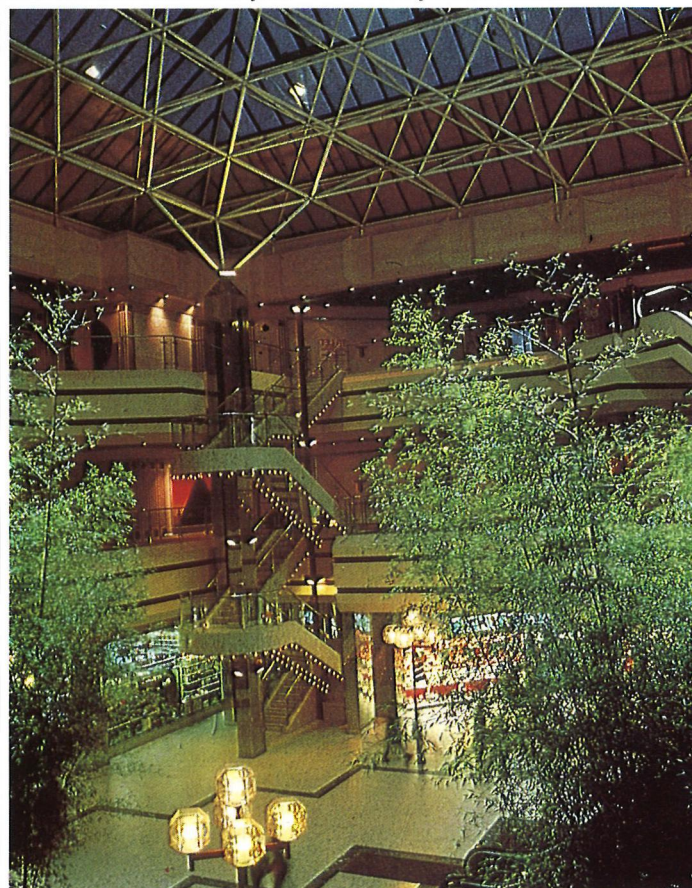
The central atrium court of the Treaty Centre at Hounslow uses powerful metal halide sources at high level to ensure growth to the three clumps of bamboos. A high level of artificial light is required in spite of good natural lighting.
